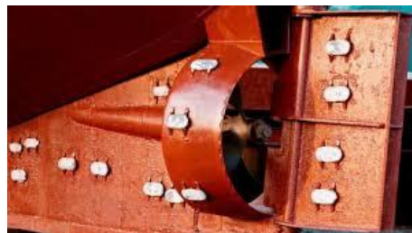
Figure 6 – Reactive Zinc blocks placed in the hull of a ship.
