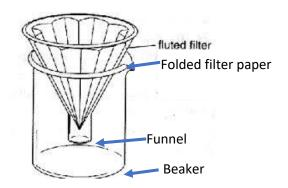
Step 6 – Pour 15 mL of acetone into the mortar with the crushed chips. Stir gently with a glass stirring rod for 5 minutes, before pouring the contents of the mortar slowly into the filter paper. Wash the chips out of the mortar and into the filter paper using the remaining 10 mL of acetone.
