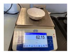
Step 2 – Place 2 large, normal chips in the evaporating dish that was weighed in step 1 and reweigh the chips and evaporating dish. Record the result.
