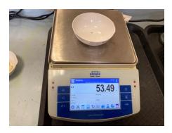
Step 8 — Transfer the contents of the beaker into the evaporating dish that was weighed in step 7 and place in a fume-cupboard overnight to allow the acetone to evaporate.
