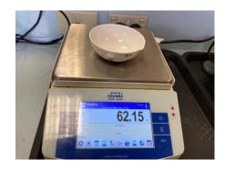
Step 2 – Place 2 large, normal chips in the evaporating dish that was weighed in step 1 and reweigh the chips and evaporating dish. Record the result.
