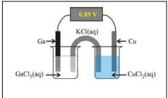
The cell potential was measured at 0.89 V, with the copper electrode gaining mass when the cell was discharging.
