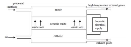
They operate at temperatures in excess of 500°C.
