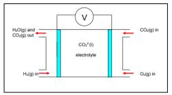
$Na_2CO_3$  as the electrolyte. Hydrogen gas is passed over one electrode and a combination of oxygen gas and carbon dioxide gas is passed over the other electrode, as shown in the diagram below. The net overall reaction is  $H_2(g) + O_2(g) -> H_2O(g)$ . There is no net gain or loss of the electrolyte.
