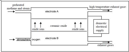
Combustion of methane drives the fuel cell. One of the half equations is given below.
