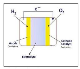
two containing the reactants and the middle one containing the electrolyte. These compartments are separated by porous electrodes that act as catalysts. Porous electrodes allow for the passage of ions through them to react with ions in the electrolyte and also allow for the conduction of electrons. An electrolyte serves to move ions from one electrode to the other.
