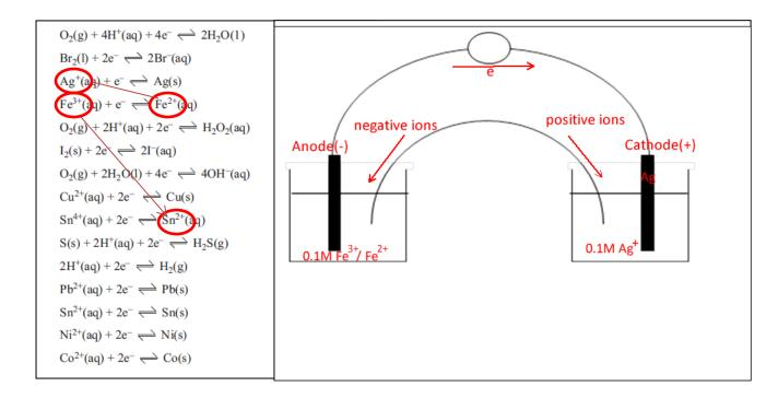
Only two solutions can undergo a spontaneous reaction with the  $Fe^{3+}/Fe^{2+}$  half cell. They are pictured above on the diagram of the electrochemical series.  $Ag^{+}$ , however, will form an electrode with a positive polarity, since reduction of the  $Ag^{+}$  ion will take place.
