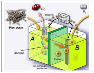
a) Which cell represents the anode? Explain The anode half-cell is "A". Bacteria consume acetic
